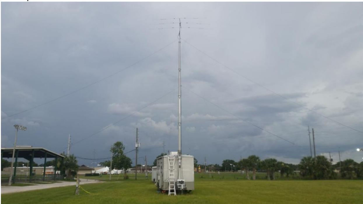
The 40, 75 meter Double Bazooka wire arrays and tri-beam antenna on top. Note the clouds (lightning capable).
