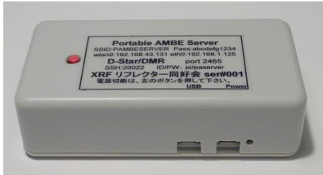
Pictured is the Portable AMBE server. Size is 9cm wide x 4.5cm depth x 2.5cm high. It can be connected to the network by WiFi or LAN connection via USB port. WiFi connection is very convenient. Two square holes are USB interface and power supply connectors. Beside the square hole, is a LED indicator which shows status of cpu inside.
