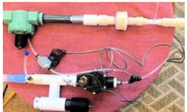
**Airway components of the emergency ventilator. [Photo courtesy of Gordon Gibby, KX4Z]**
