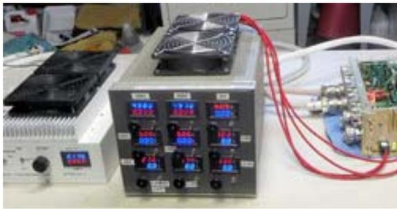
Part of the ARISS InterOperable Radio System -- the multi-voltage power supply -- being put through its paces during one of its many NASA tests. [Photo courtesy of ARISS]
